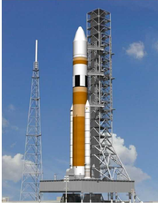
Figure 5.—Ares V and Altair on the launch pad next to the launch umbilical tower.
