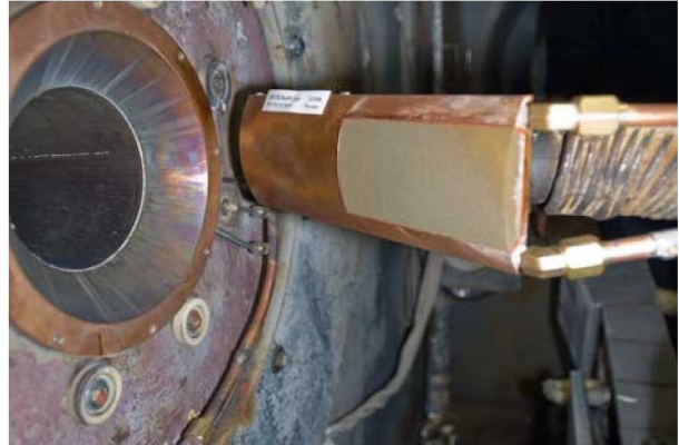
Figure 5 Swept Cylinder mounted in the arc jet.
