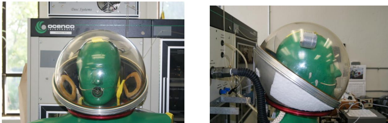
Figure 9. Mark III open configuration helmets installed onto test stand.
