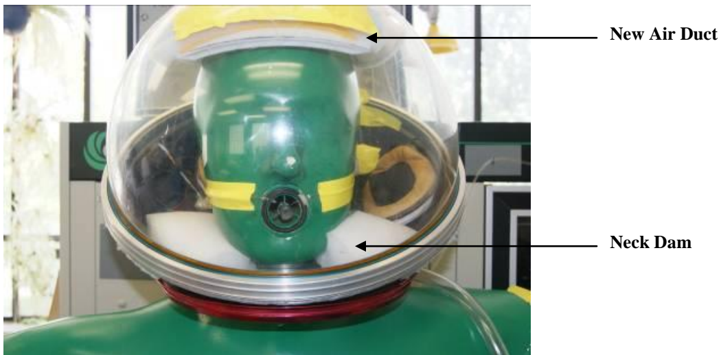
Figure 22. Mark III open helmet with new air duct and neck dam.
