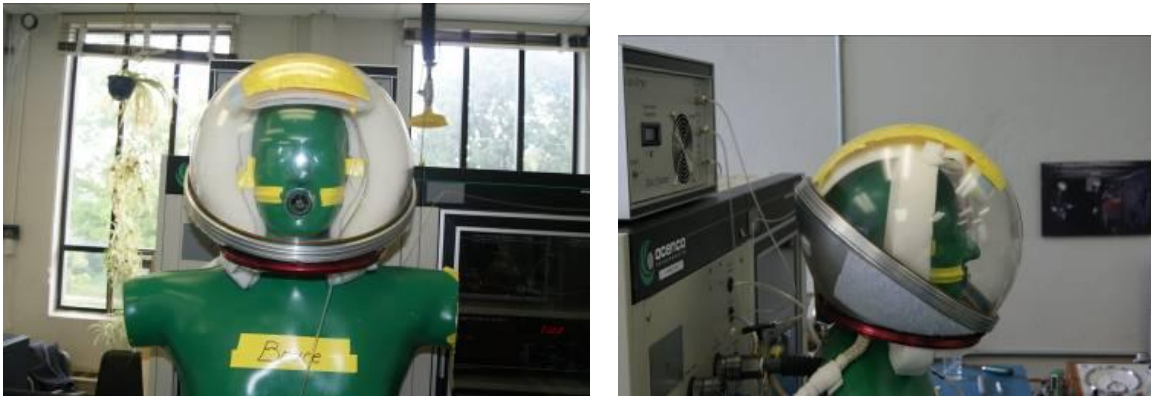
Figure 10. Mark III Conformal helmet installed onto test stand.
