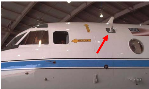
Figure 6. WP-3D with TAMDAR Installed.
