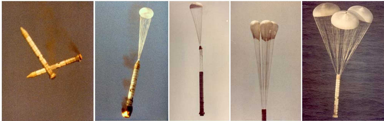
Fig. 4. Early Cast Glance Support of the Shuttle Program (circa 1980-90s). Shuttle Rocket Booster (SRB) Parachute Deployment
