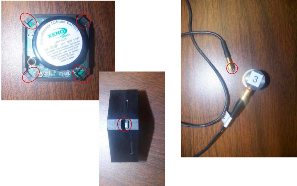
Figure 7.3-8. a) DIDS Body Showing a Missing Jack (circled in red). b) DIDS Showing Four Missing Jacks (circled in red). c) Cable with AE Sensor and DIDS Jack (circled in red).
