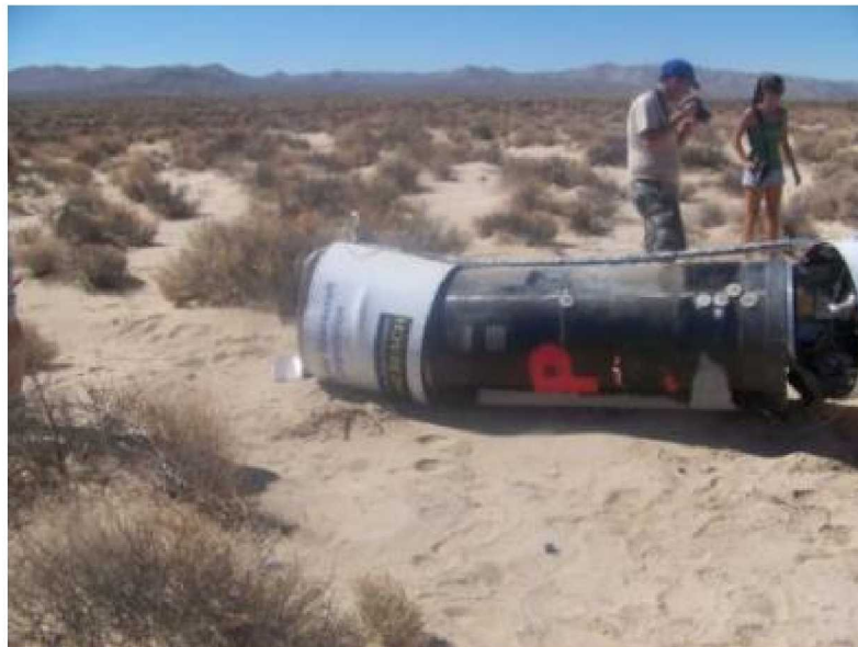
Figure 7.3-5. P-9 Rocket Crash Site Showing Vehicle Forward Section
