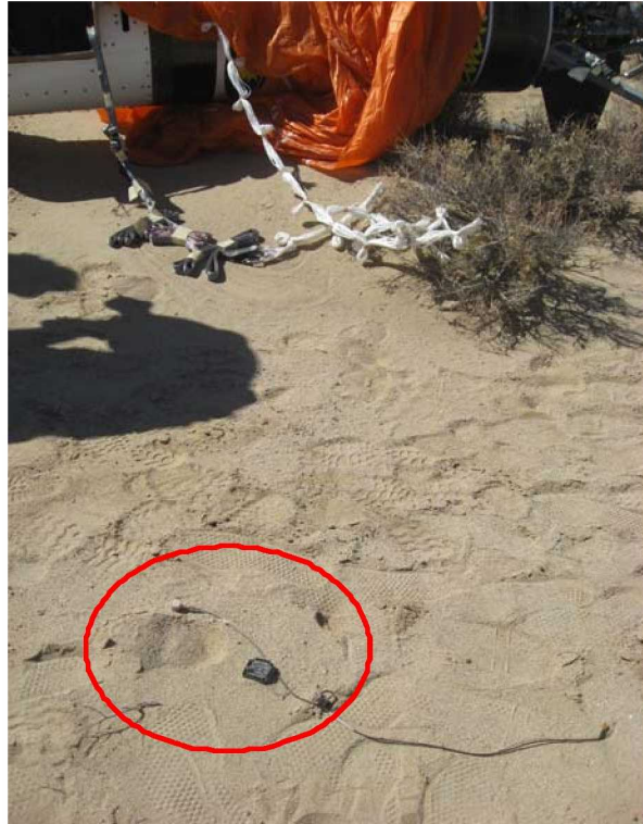
Figure 7.3-7. P-9 Crash Site with Ejected DIDS, Sensor and Cable
