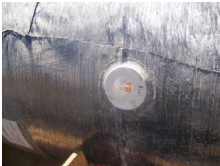
Figure 7.3-6. P-9 Rocket LOX Tank Showing Longitudinal Crack
