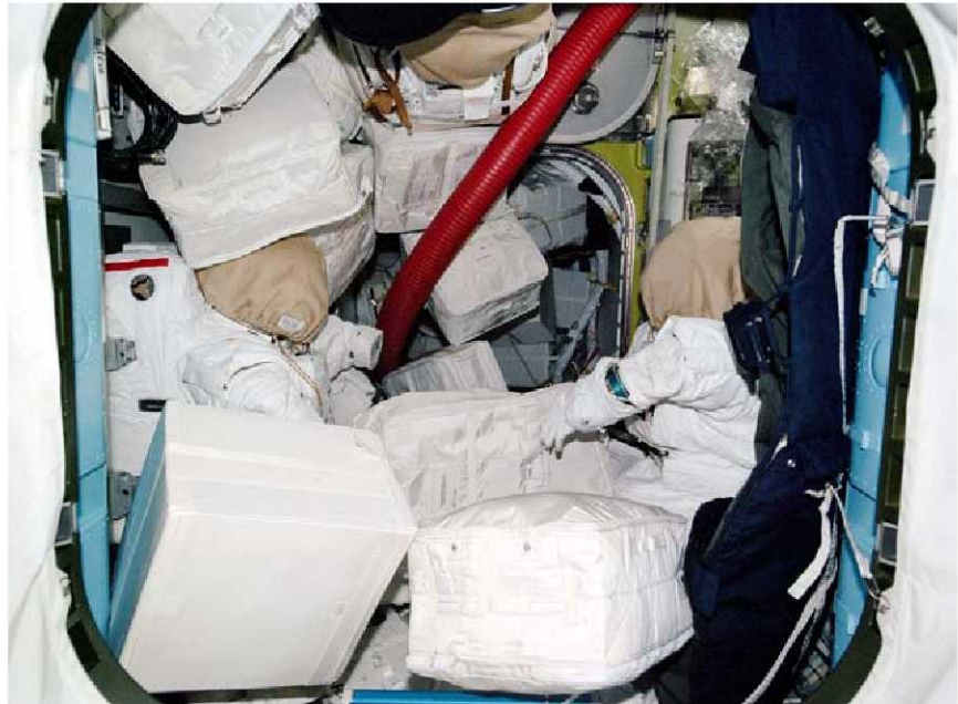
Figure 5. Interior of the Node1 module during the UF-1 docked mission, exhibiting crowded stowage detrimental to cabin airflow. Image Credit: NASA
