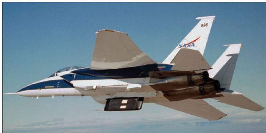
Figure 1. Two Very-High-Speed Digital Video Cameras are mounted in forward and aft camera pods, respectively, on the F-15B Research Testbed aircraft. The cameras are positioned to obtain photogrammetric data of simulated space-shuttle external-tank thermal-insulation foam debris released from a fixture under the centerline of the aircraft at flight speed up to Mach 2.
