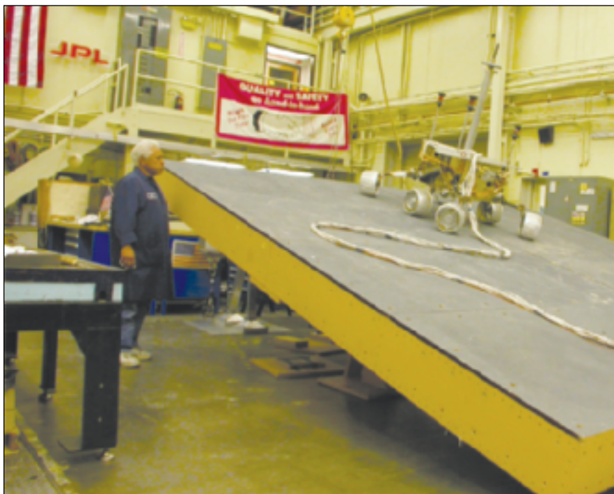
A Model Robotic Vehicle was driven over 25-cm obstacles on simulated terrain at a tilt of 20°.
