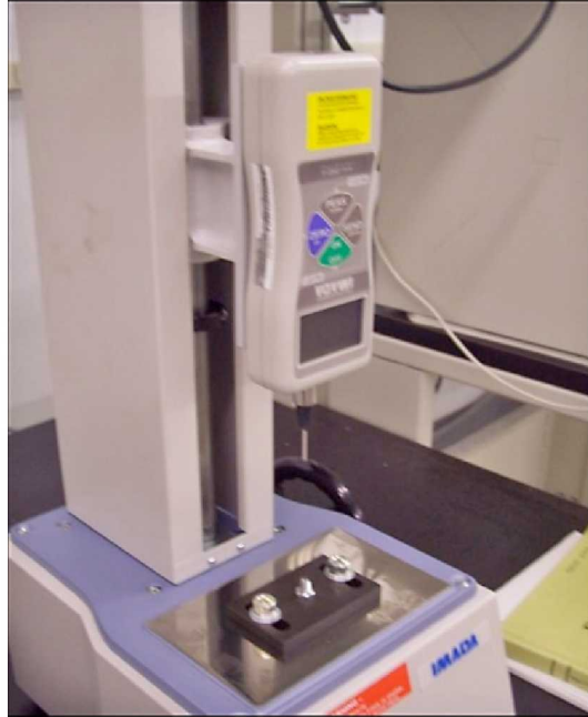
Figure 9.—Force Gauge with penetrating pin installed mounted onto hand wheel test stand.
