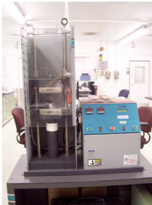
Figure 28.—Carver automatic hydraulic press.
