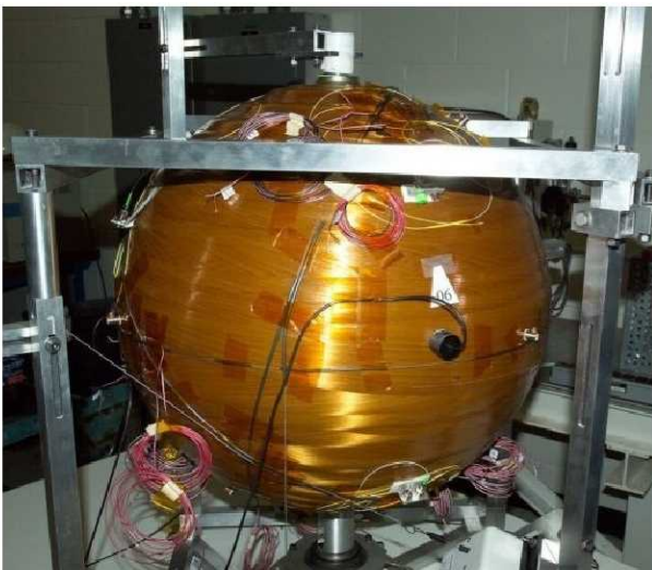
Figure 7. Typical Kevlar-epoxy vessel pre-test instrumentation
