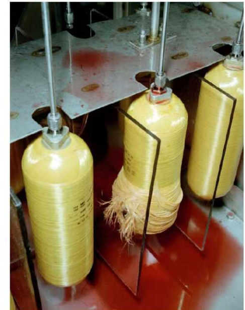
The first flight-rated COPV stress rupture tests were at WSTF
