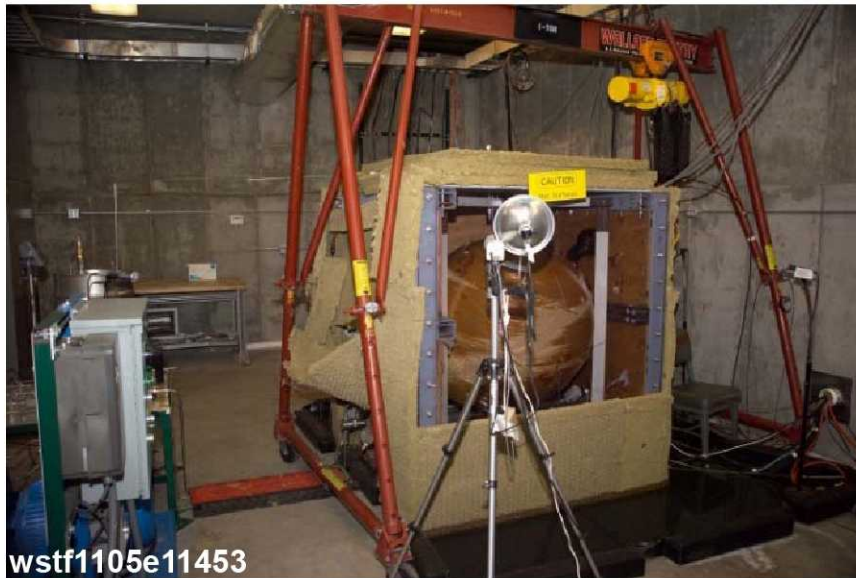
Kevlar vessel upon completion of stress rupture test
