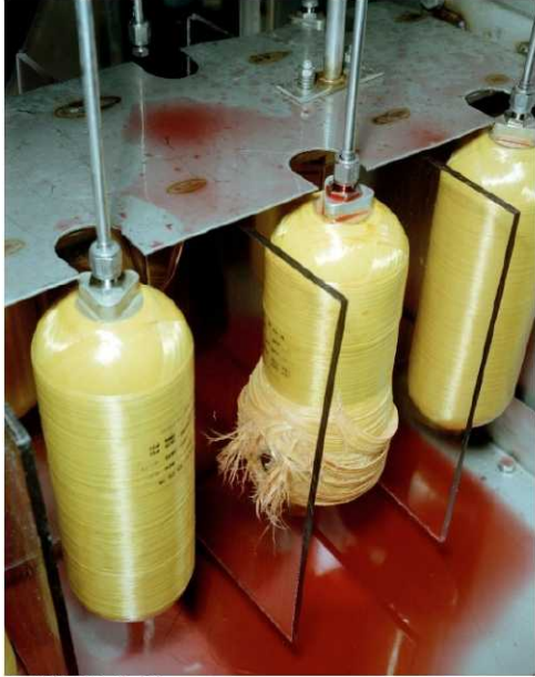
Figure 1. The first flight-rated COPV stress rupture tests were at WSTF
