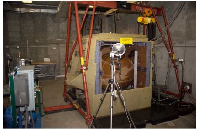
Figure 8. Kevlar vessel upon completion of stress rupture test
