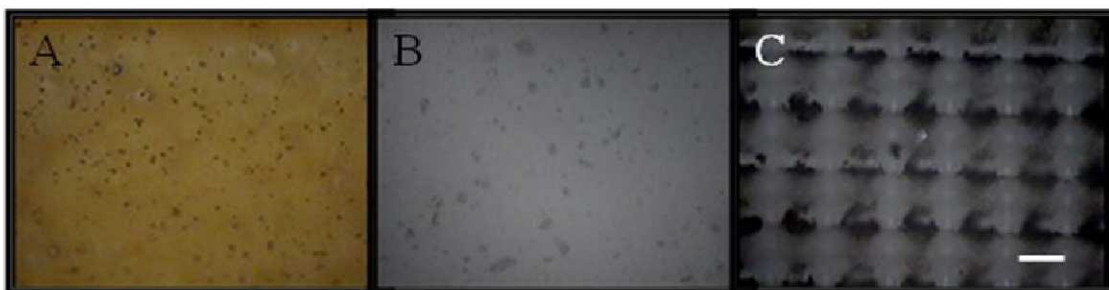
Figure 9. Sonic wand adhesion testing indicated that the polyimide surface (A) retained a greater number of particles than the copoly(imide siloxane) surface both before (B) and after laser ablation patterning (C). The lunar simulant particle retained on the laser ablation patterned surface can be seen near the center of the image. The scale bar is 25 \mu\text{m} .
