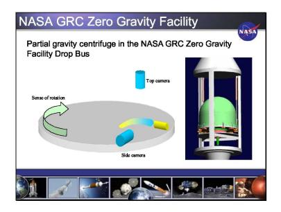
To study the partial gravity effects on ground, a centrifuge was developed for use in drop tower experiments. It consists of a turntable and a chamber dome (since the drop tower is evacuated before a drop). Note that the rotating chamber needs time to spin-up all the internal gas so that it rotates as a solid body. Only then can the analogy of centrifugal force to gravitational force be made.
