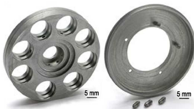
Figure 9. Mo-41%Re parts machined from arc-cast material for AMTEC system.
