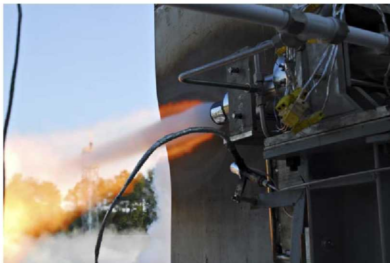
Figure 4 – Workhorse Gas Generator testing at MSFC
