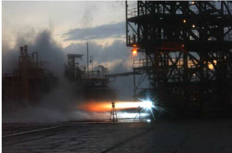
Figure 3 – Subscale Main Injector testing at MSFC
