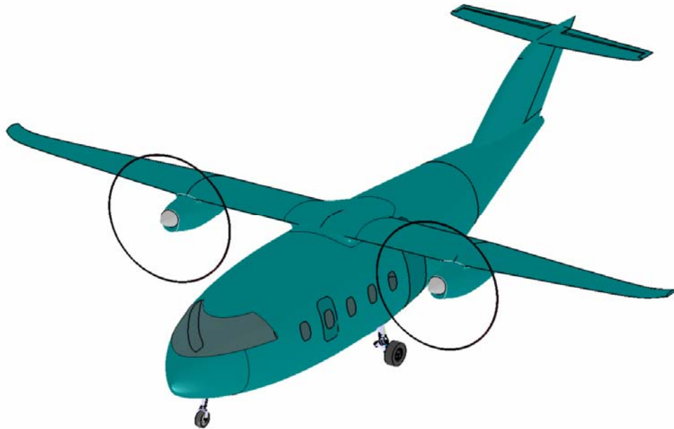
Figure 167. Advanced 20 Passenger Turboprop Airliner for Y2035
