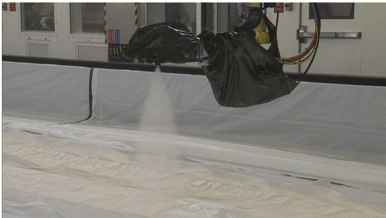
Figure 5. Initial acceptance testing of the SOFI robotic spray booth in December 2009.
