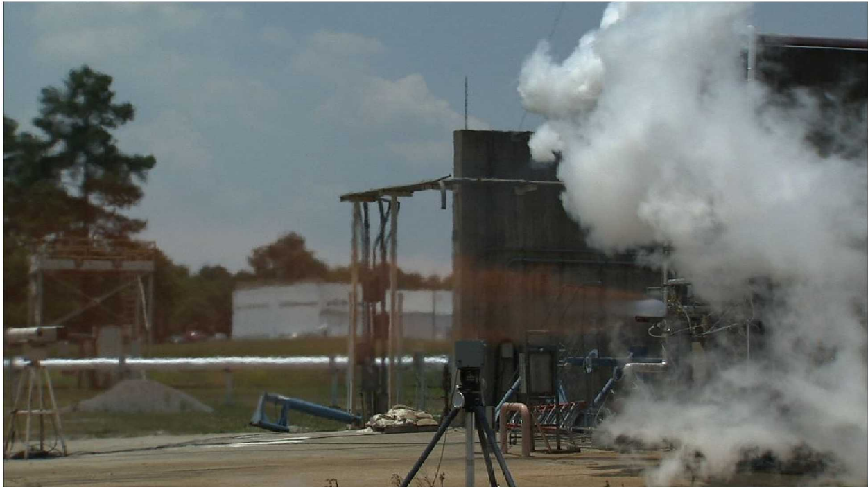
Figure 3. Workhorse gas generator testing at MSFC's Test Stand 116.
