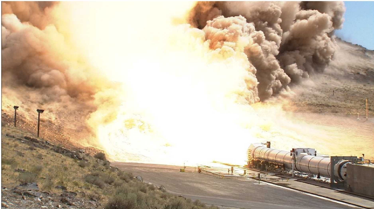
Figure 1. Static test firing of Development Motor 1, September 2009.
