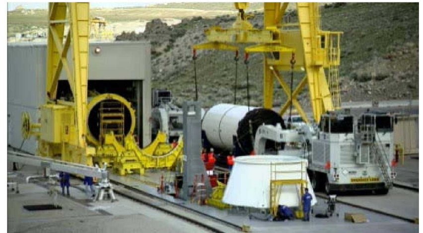
DM-1 Installed at TS 97
