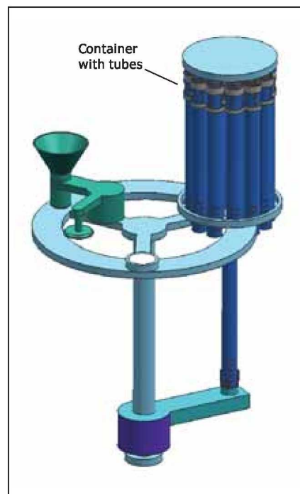
Figure 2: Containerization System includes loading, heating/sealing, and storage stations.
