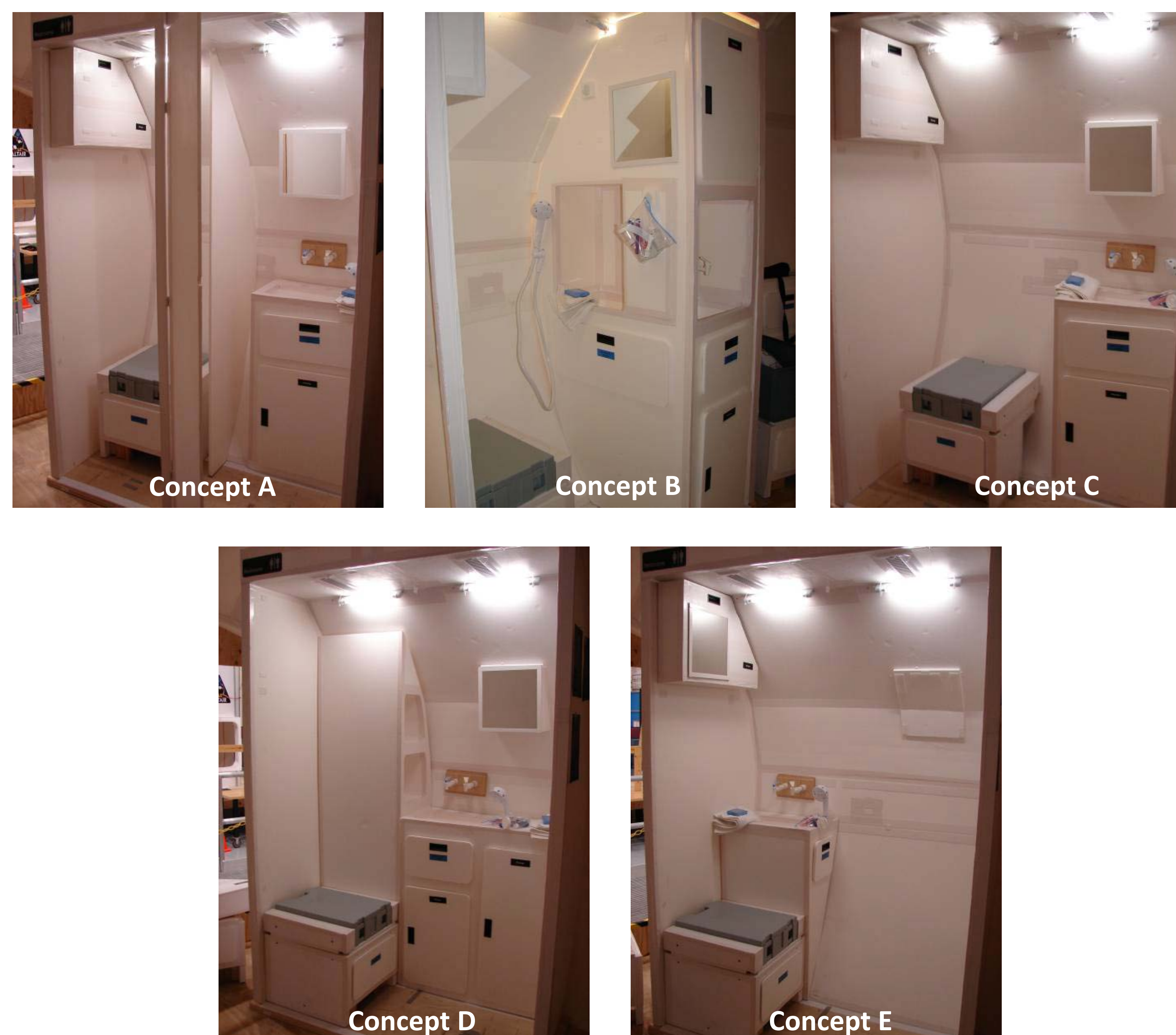
Figure 3. The five wet-bath concepts evaluated during the current study. Notice how some of the designs exploited more stowage space, while others had more usable space.
