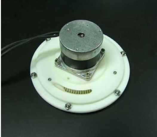
(a) Blower With Off-the-Shelf Motor and With Inlet and Exit Diffusers Removed
