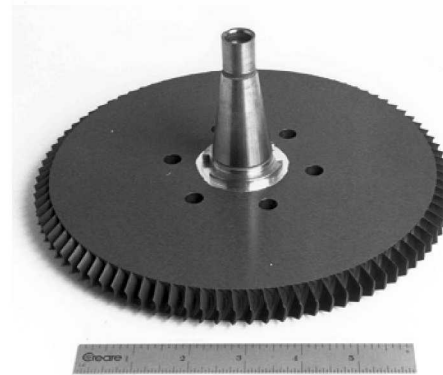
(b) Impeller From a Regenerative Compressor
