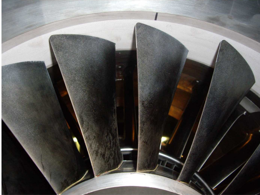
Figure 3.—A metal foam OTR treatment with perforate cover sheet installed in the ADP model.
