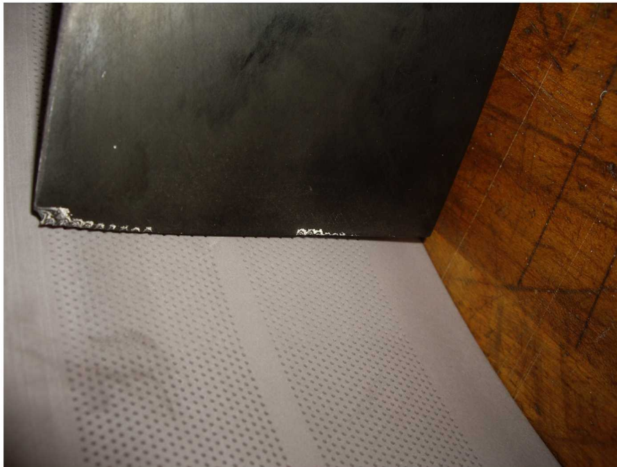
Figure 6.—Damage on the composite blade which coincides with the holes in the perforate covering the metal foam OTR treatment.
