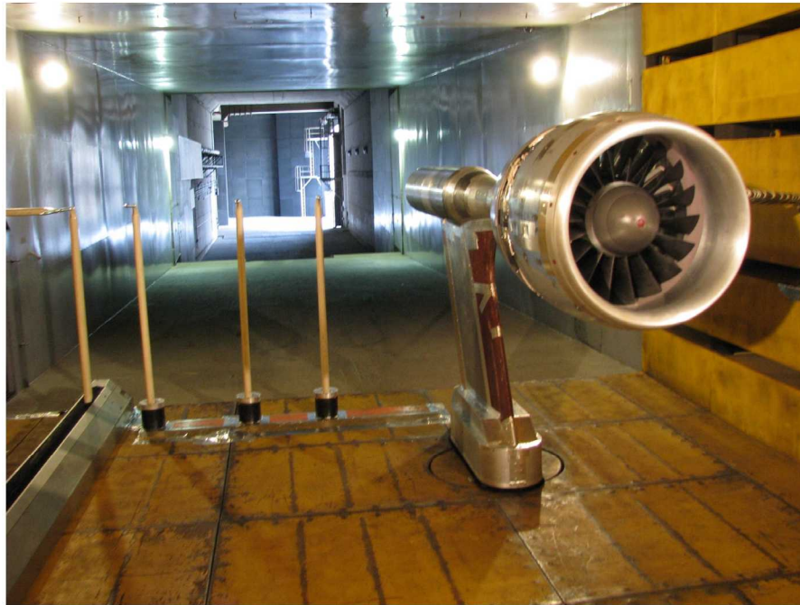
Figure 1.—The Advanced Ducted Propulsor model as installed in the NASA Glenn Research Center's 9- by 15-Foot Low-Speed Wind Tunnel. Microphones are visible at left.
