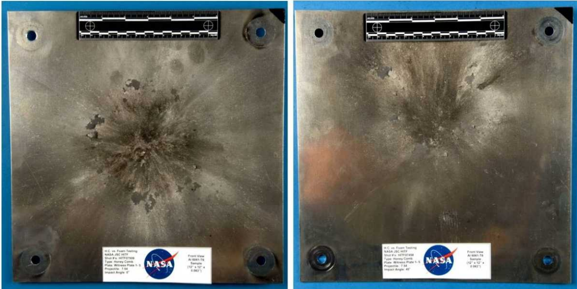
Figure 13: Comparison of impact damages in the DL-H target rear wall impacted by 0.754 cm diameter Al 2017-T4 spheres at ~6.9 km/s with normal (left) and oblique ( 45^\circ , right).
