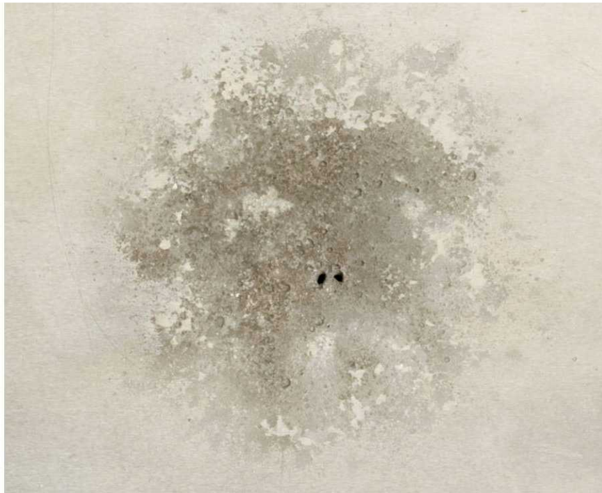
Figure 26: Solid fragment craters on the DL-F rear wall at high impact velocities (0.877 cm diameter Al2017-T4 sphere at normal incidence with 6.76 km/s).
