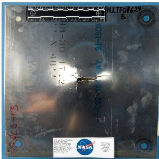
Figure 11 (cont): Comparison of impact damages in the DL-H (left) and DL-F (right) targets impacted by a 0.833 cm diameter Al 2017-T4 sphere at 6.83 \pm 0.09 km/s and 0^\circ . From top to bottom: rear wall (front view), rear wall (rear view).
