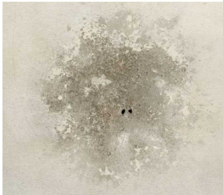
Figure 15: Melted aluminum deposits and solid fragment damage of the DL-F rear wall impacted by a 0.717 cm diameter projectile at 3.29 km/s with normal incidence (HITF08595).
