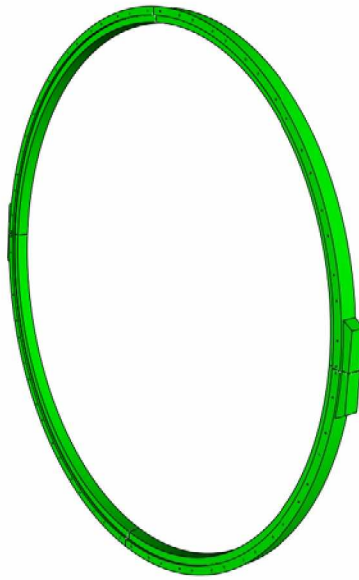
Figure 4.8. Attachment ring shown as an entire part. To simplify the analysis, only a quarter of the geometry was used for the finite element analysis.
