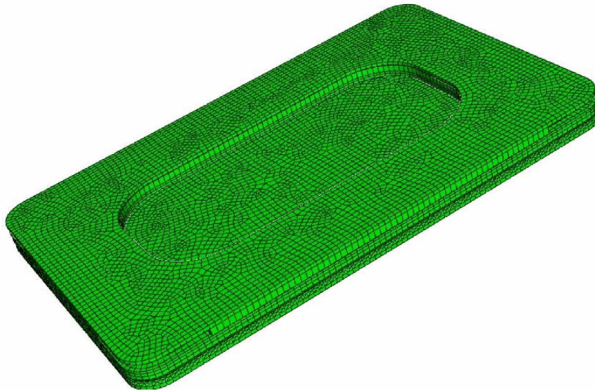
Figure 4.11. Fully assembled geometry and finite element mesh used in the habitat's window analysis.
