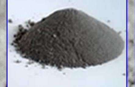
**JSC-1A** •Developed at Johnson Space Center Second version (JSC-1 was the predecessor) Designed to match Apollo 14 regolith sample 14163 (mixture between a highlands and mare composition)
