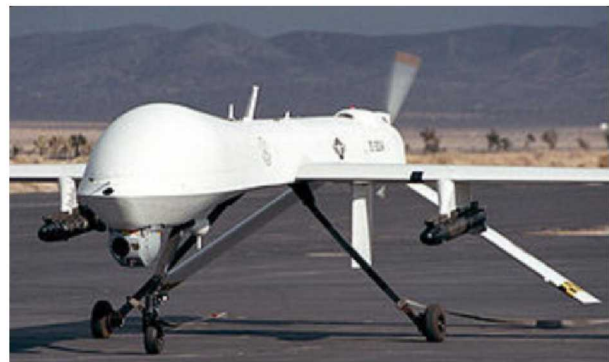
Fig. 8 Rotax 914, a four-cylinder, four-stroke, 101-horsepower engine, the same engine type commonly used on snowmobiles, rotates the Predator's two-blade, variable-pitch pusher propeller (Valdes, R., 2009; Rotax Aircraft Engines, 2009; and Thielert Aircraft Engines, 2009)
