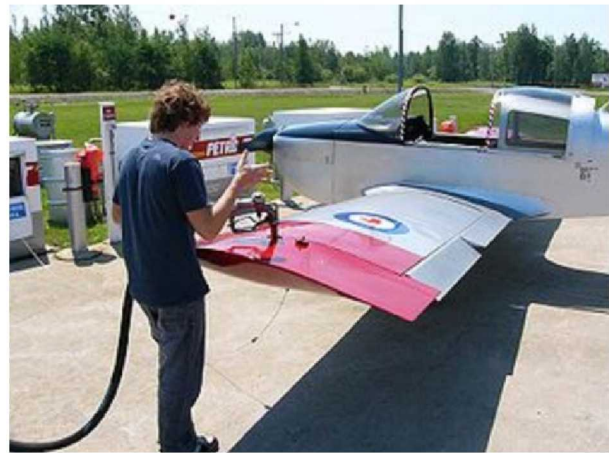
Fig. 7 An American Aviation AA-1 Yankee being refueled with 100LL Av-gas (Wikipedia, 2009g)
