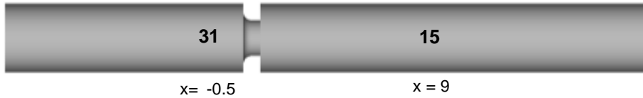
Figure 14. Orifice Domain Showing location of the Upstream Probe(31) at x=-0.5 and Downstream Probe(15) located at x=9.
