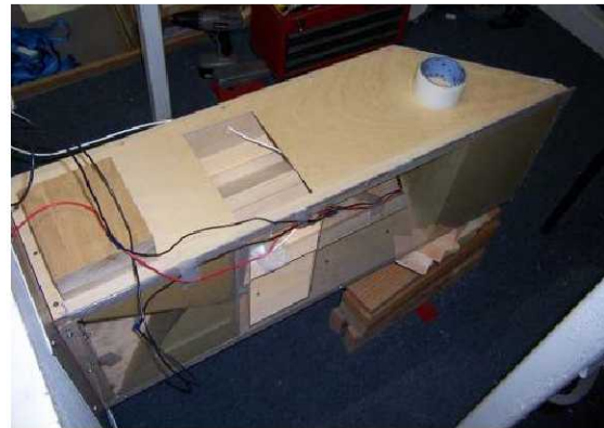
Figure 9. Initial functional exhaust duct (wood and melamine) functional mockup.
