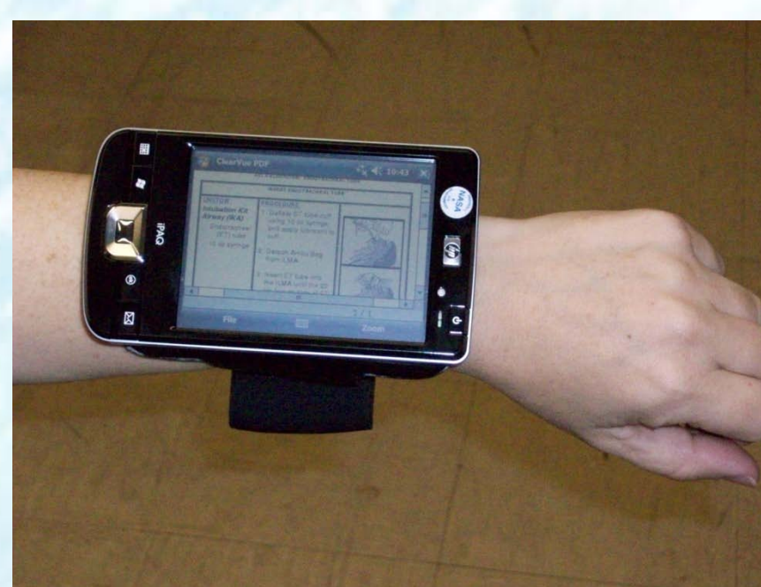
Procedure displayed on wrist mounted PDA
