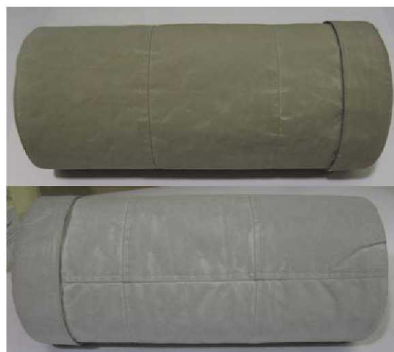
Figure 9. Comparison of hue between simulant types. The JSC-1 simulant turned test articles a darker shade of gray than the NU-LHT-2C simulant, as shown above. Test articles pictured are Test Article #2 (top) and Test Article #8 (bottom), both fabricated from the W.L. Gore 4 Harness Satin material.
