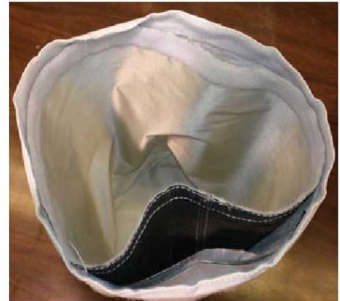
Figure 2. Cover layer lay-up. Lay-up used for all cylinder cover layers. From inside to outside: one layer neoprene coated nylon rip-stop, five layers aluminized Mylar, one layer candidate fabric.
