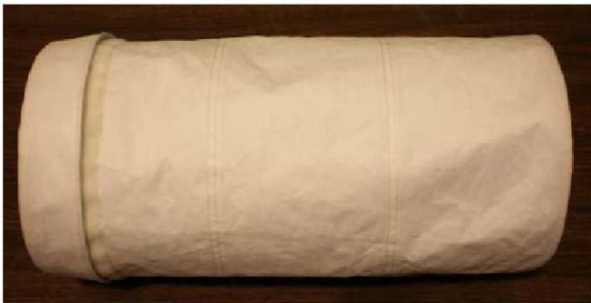
Figure 3. Example fabric test cylinder. Fabric test cylinder before tumble test.
