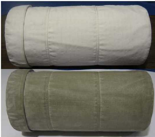
Figure 4. Test article pre-/post-test photos. Photographs of Test Article #1, the Orthofabric test cylinder, before (top) and after (bottom) tumbling for 8 hours with JSC-1 simulant.
