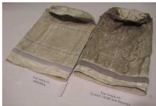
Figure 7. Comparison of Orthofabric and Tyvek post-testing. As shown above, the Tyvek test article displayed much more degradation post-testing than other fabrics, such as the Orthofabric.
