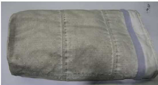
Figure 5. Test article post vacuuming. Test Article #1, the Orthofabric test cylinder, after being vacuumed to remove simulant.
