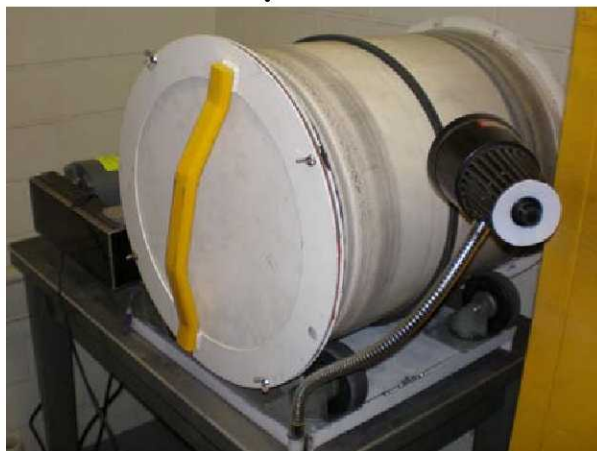
Figure 1. Rotary Drum Tumbler. Drum tumbler was used to simulate 8-hour EVA with each test article.
