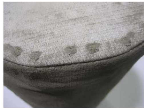
Figure 6. Damage on test article end-cap. One of the common themes across test articles was abrasive wear on the end-caps. The photo above displays wear as seen on the Test Article
