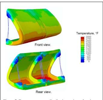
Figure 7. Entry temperature distribution at time of peak temperature.
