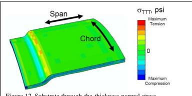
Figure 12. Substrate through-the-thickness normal stress distributions on the lower-apex local model at the coating-substrate interface for the best-estimate stress-free temperature for the uniform elevated-temperature condition.
