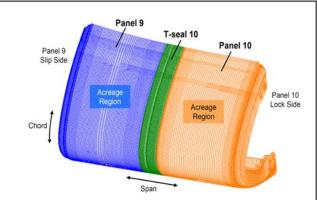
Figure 2. Integrated model of Panel 9, T-seal 10, and Panel 10.
