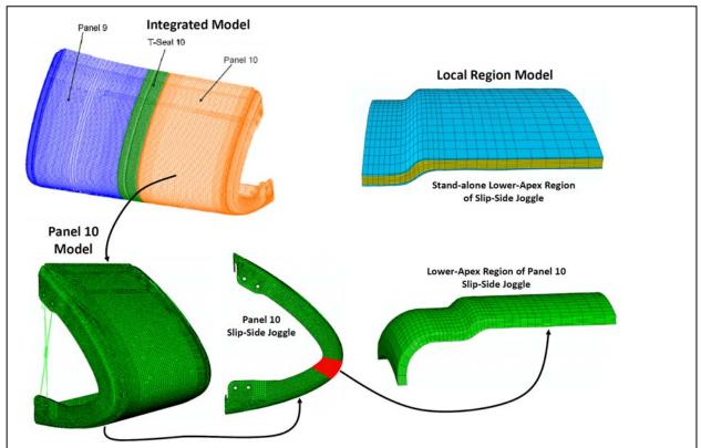
Figure 3. Three different configurations to be analyzed – Integrated model, single-panel model of Panel 10, and local region model.
