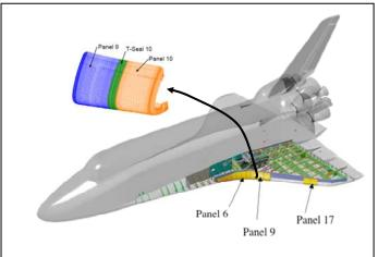
Figure 1. Space Shuttle Orbiter and wing-leading-edge cutaway view.
