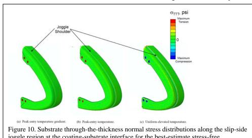
joggle region at the coating-substrate interface for the best-estimate stress-free temperature for three thermal loading conditions.
