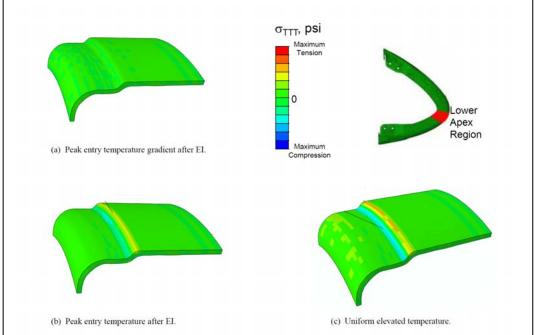
Figure 11. Substrate through-the-thickness normal stress distributions along the lower-apex region of slip-side joggle region at the coating-substrate interface for the best-estimate stress-free temperature for three thermal loading conditions.
