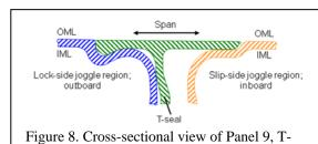
Figure 8. Cross-sectional view of Panel 9, T seal 10, and Panel 10.
