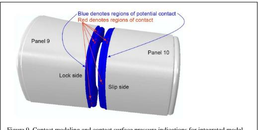
Figure 9. Contact modeling and contact surface pressure indications for integrated model.
