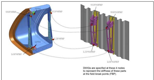
Figure 6. Connections between field-break points (FBP) on panel assembly and WLE front spar.
