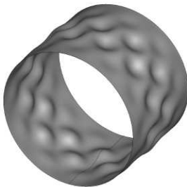
(d) shape and normal deformation for intermediate buckling configuration
