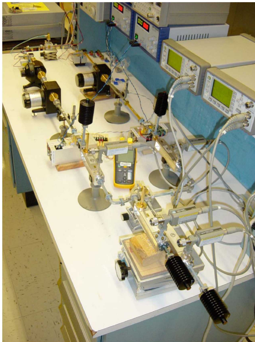
Figure 8.—Laboratory bench top 2-way MMIC power combining test circuit.
