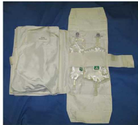
Figure 6. Water pack opened showing silver and iodine standard solutions.
