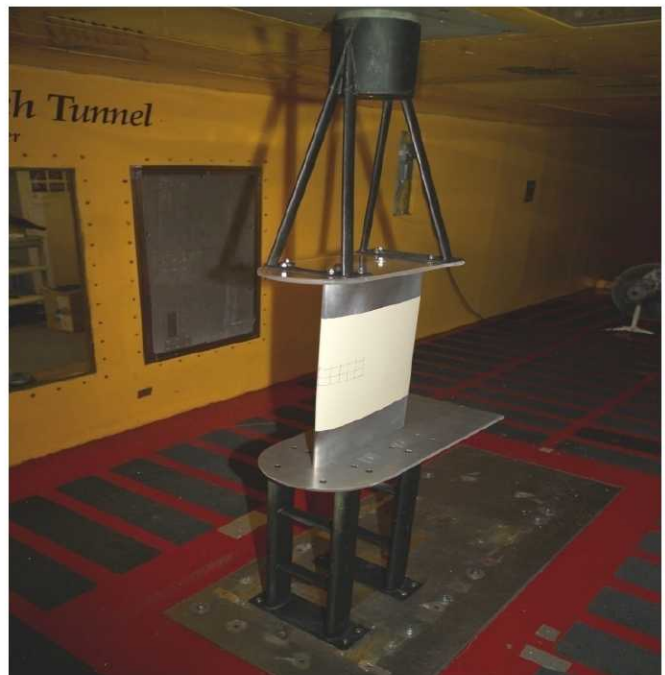
Figure 3.—35.6-cm chord model in the IRT test section.
