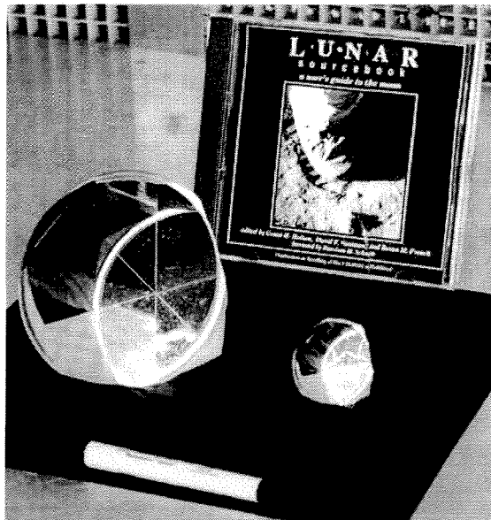
Figure 7: A 10 cm solid cube corner reflector was recently qualified for the lunar environment. Also shown for comparison is a 3.8 cm Apollo engineering model cube corner [11]. Photo courtesy of Douglas Currie.
