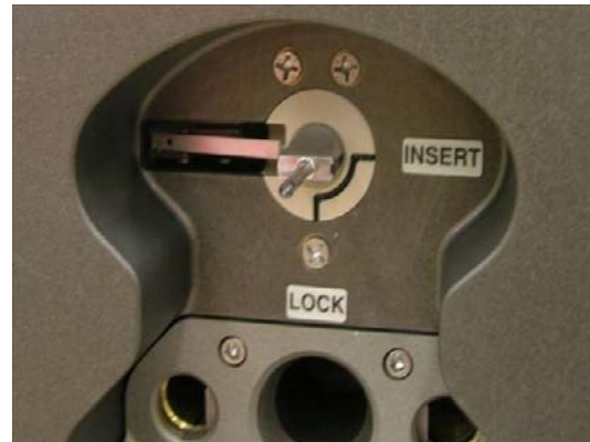
Figure 12. Behind the Beverage Adapter, PIP Switch
