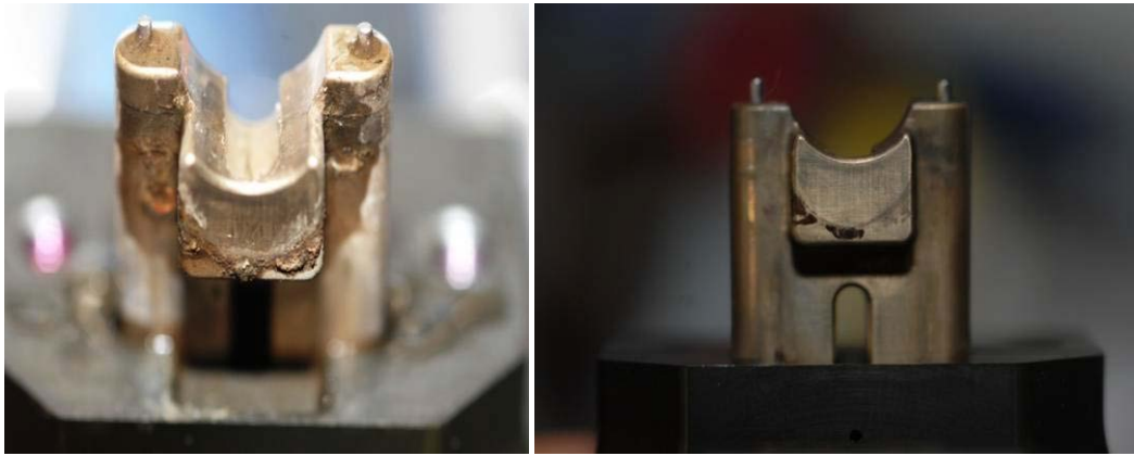
Figure 17. Precleaning (left) Postcleaning (right): On-orbit Photos of the Food Residue/Corrosion on the Slide Assembly Internal to the Beverage Adapter
