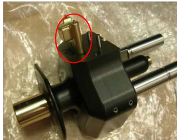
Figure 16. Beverage Adapter Opened, Showing the Slide Assembly (RED)
