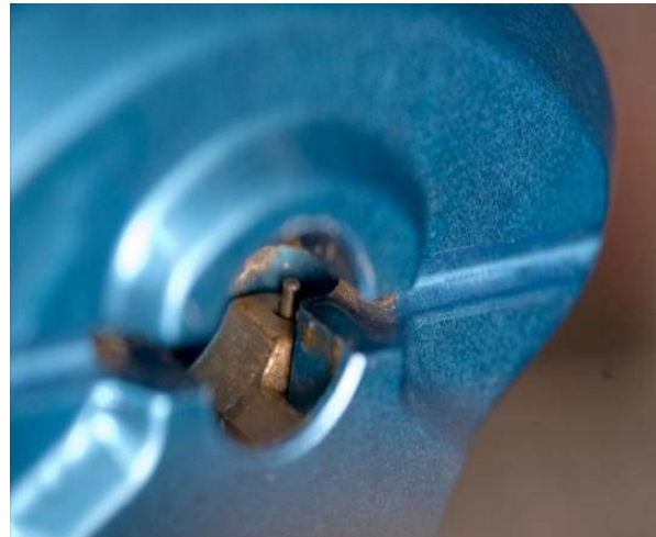
Figure 15. On-orbit photo of PWD Package Insert Port with Food Residue/Corrosion within the Beverage Adapter the PIP Switch with Tape
