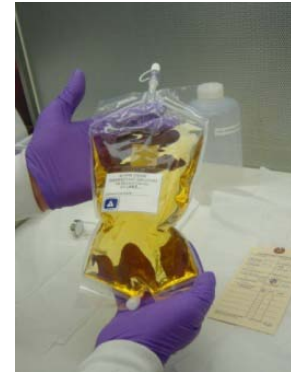
Figure 6. Teflon Bag filled with 40 ppm I_2
