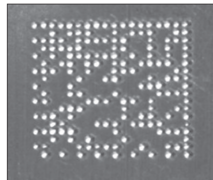
Figure 2. A Data-Matrix Symbol marked with low contrast using a dot peen process on a smooth aluminum target was imaged in the prototype reader at a viewing angle 15° off the perpendicular to the target surface.
