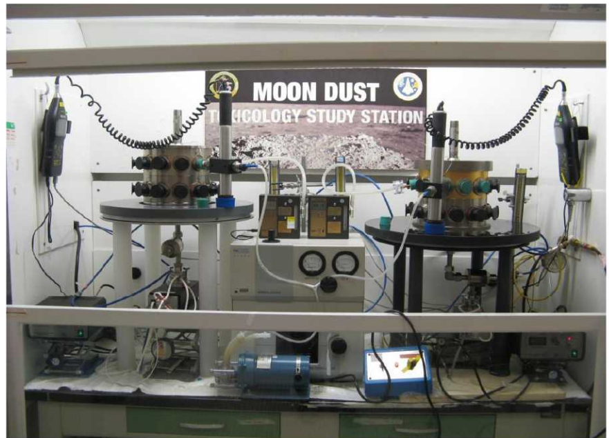
Figure 16. Nose-only inhalation exposure chamber systems, each equipped with a Vilnius Dry Aerosol Generator and a cyclone.
