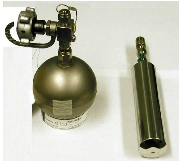
Figure 2. Grab Sample Container (GSC) from L to R: Original model, New Model
