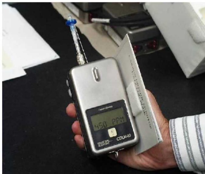
Figure 5. Carbon Dioxide Monitor (CDM)
