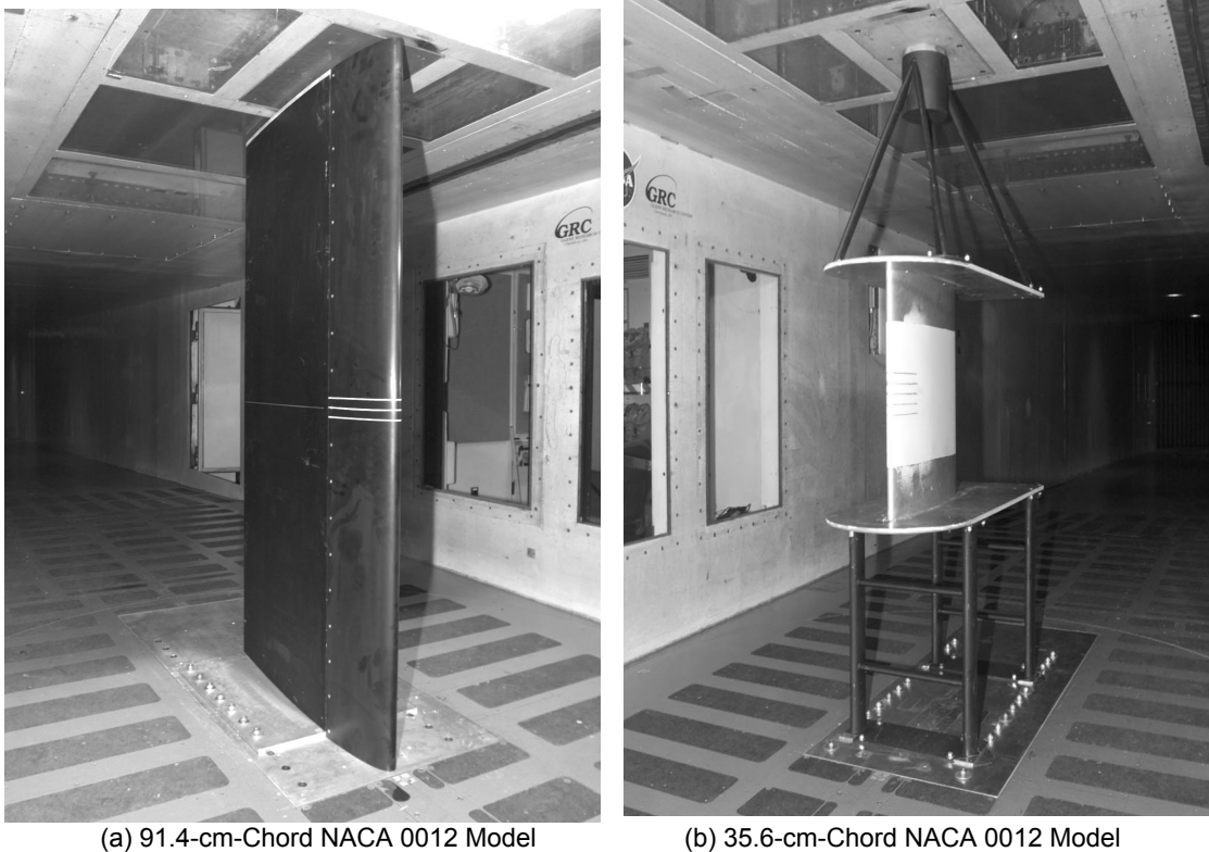
Figure 1.—Models installed in IRT test section.
