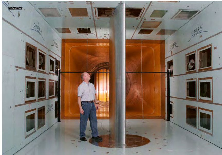
Figure 2. Photograph of the Full-Scale NACA 23012 Airfoil Model Installed in ONERA F1 Wind Tunnel Test Section
