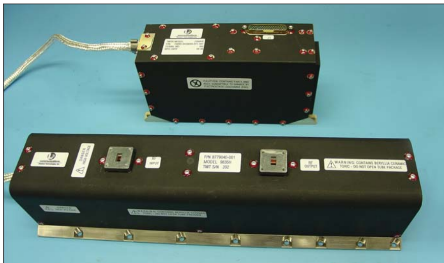
A K-Band 40-W TWTA is shown here for the Lunar Reconnaissance Orbiter Mission.
