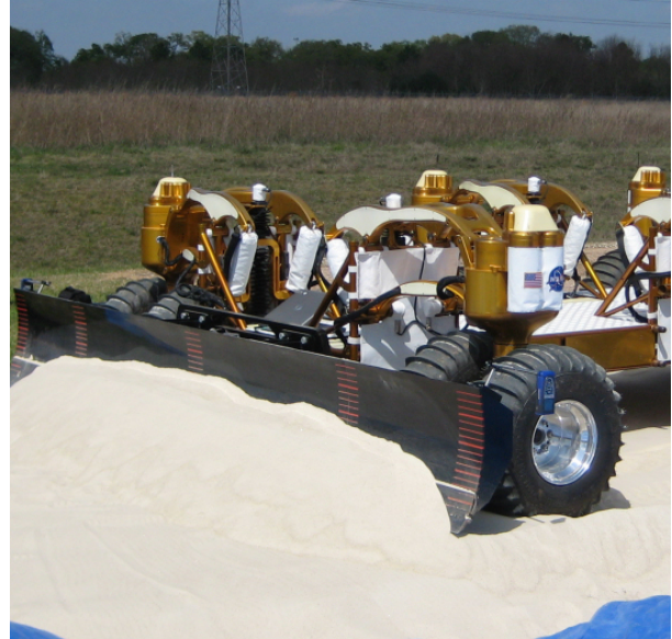
Figure 4.—Vehicle pushing GRC-1 soil at the JSC test site in May 2008.
