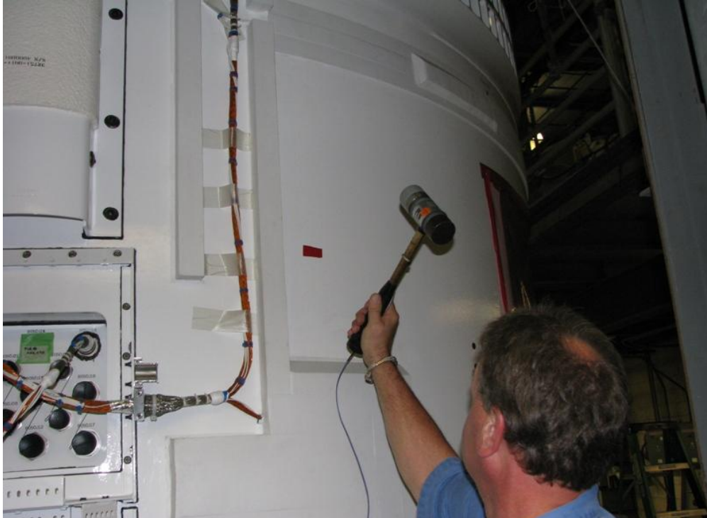
Figure 27. Exterior impact 84" up from shims at ~FTS location and 65°(56R-)
