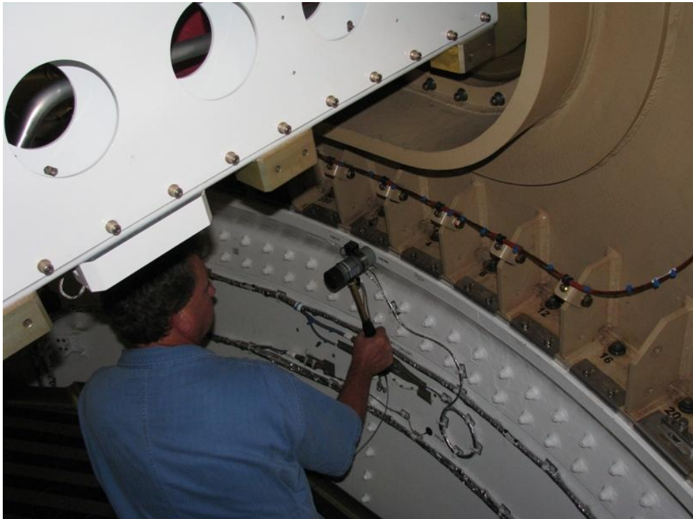
Figure 28. Impact from inside at top of frustum and 0° (57R)
