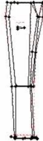
Figure E.4. Stack 2 nd Bending at 16.35 Hz
