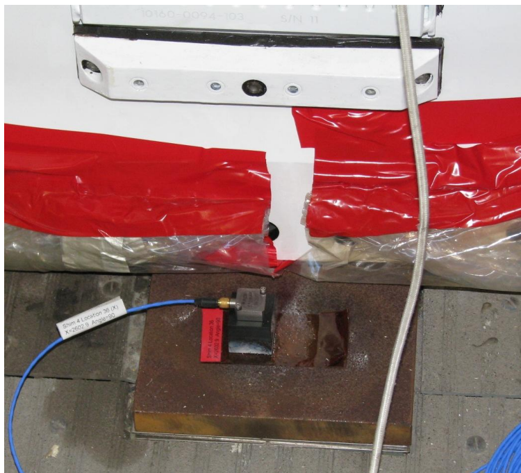
Figure 9. Shim plate 4, Accelerometer locations 36
