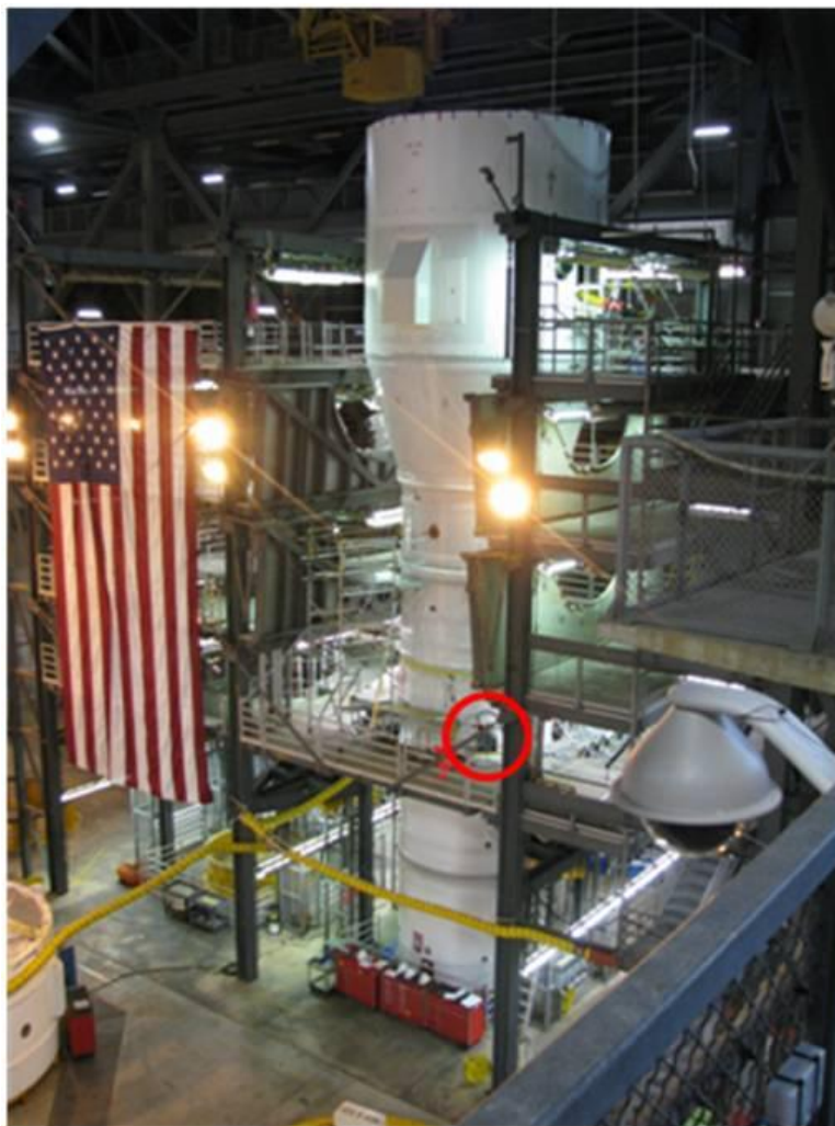
Figure 7. Stack 1 modal test setup with shaker 2 circled in red
