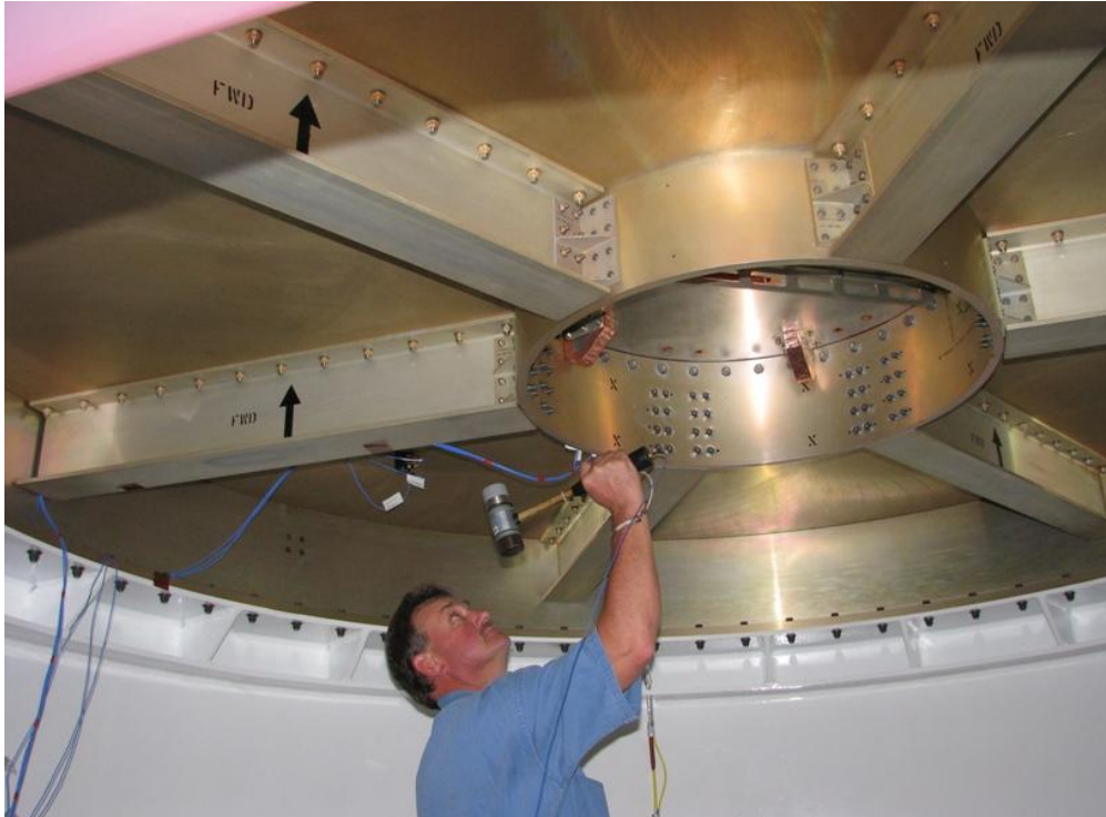
Figure 23. Impact on FSAM base plate beam at 120° (53X-)
