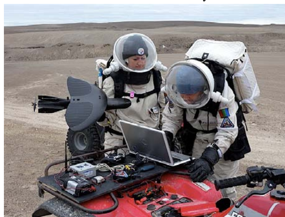
Fig. 17: Joe and Kristine preparing to launch the UAV from Maveric Flats. The control laptop sits on a platform Joe built as a power converter from the ATV battery to the laptop.
