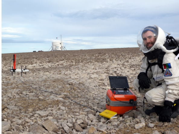
Figure 2: Brian Shiro takes some TDEM soundings with the FMARS habitat in the background.
