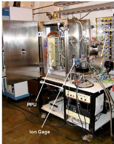
Figure 9.—Photograph of the PPU installed in GRC's VF14.
