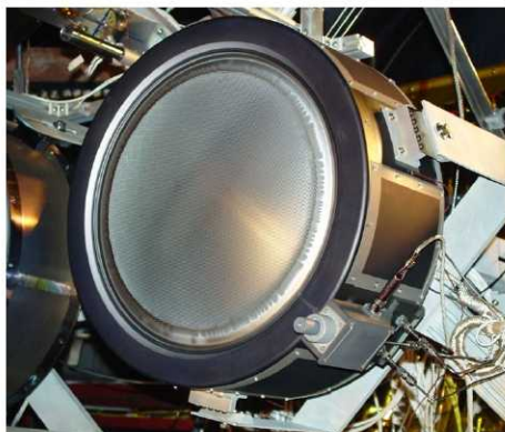
Figure 1. Photograph of the NEXT PM1R ion thruster.
