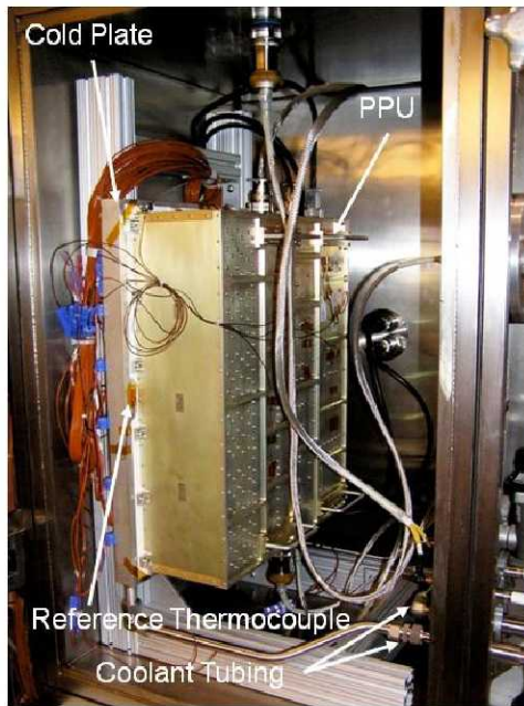
Figure 12.—Photograph of the PPU mounted on its cold plate. The reference thermocouple location is also shown.
