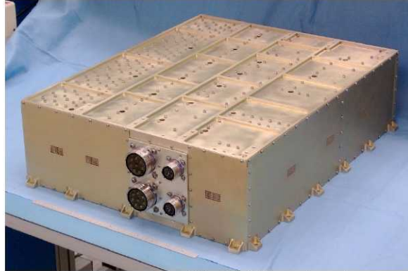
Figure 6.—Photograph of the NEXT engineering model PPU.
