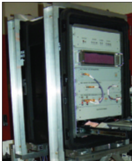
The TDS RF Design consists of a receiver rack drawer, a frequency synthesizer rack drawer, and an upconverter/downconverter.
