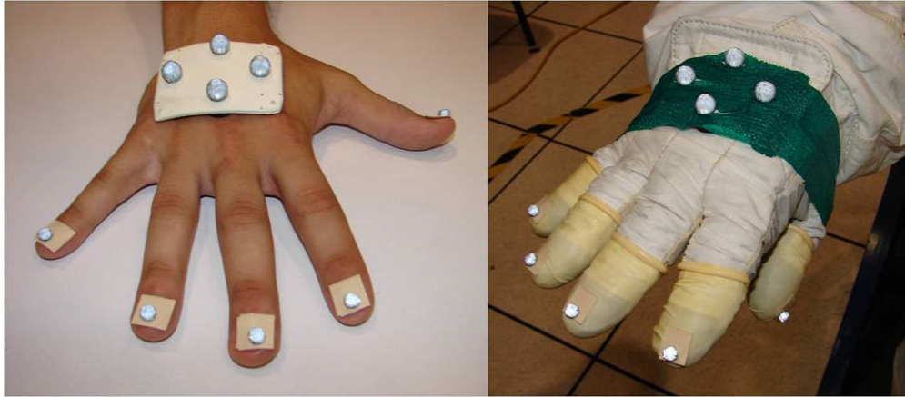
Figure 4. Example of Markers on an Ungloved and Gloved Hand
