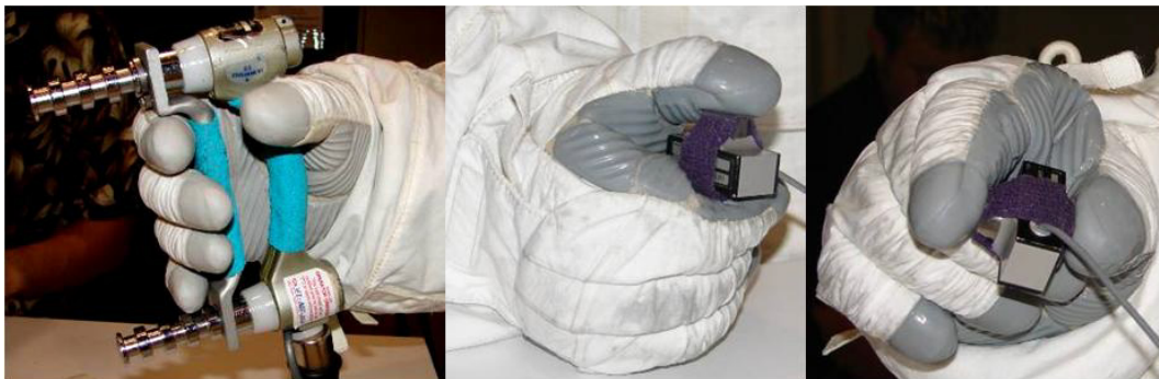
Figure 3. Grip (Left), Key Pinch (Center) and Pulp Pinch (Right) Strength Testing
