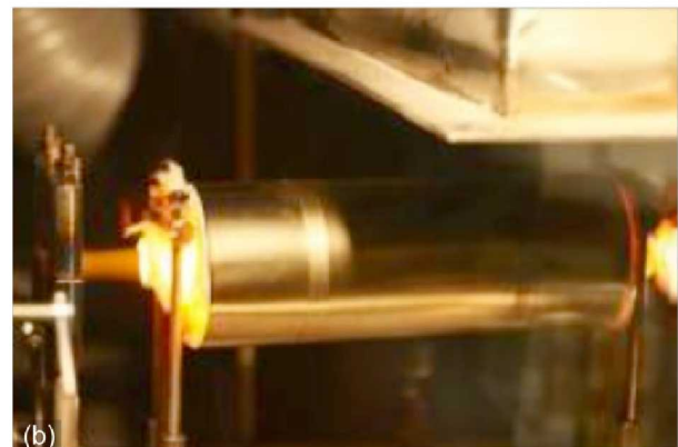
Figure 1.—Mach 0.3-1.0 high velocity burner erosion rig. (a) The burner rig for the coating erosion testing. The insets show the burner nozzle under test operation of Mach 0.9. (b) The burner rig coating erosion testing for coating erosion model validation. The burner and duct system can significantly improve the flow uniformity and erodent velocities for the erosion testing.
