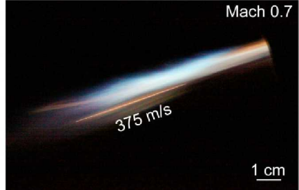
Figure 4.—Ducted rig particle velocity analysis and measurements for 27 \mu\text{m} size particles. (a) CFD modeling. (b) Burner particle velocity measurements.
