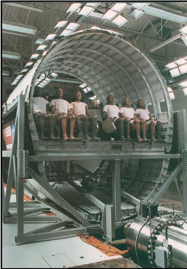
Figure 2: HYGE Crash Simulator (Actuator in lower right; Test Article at center)
